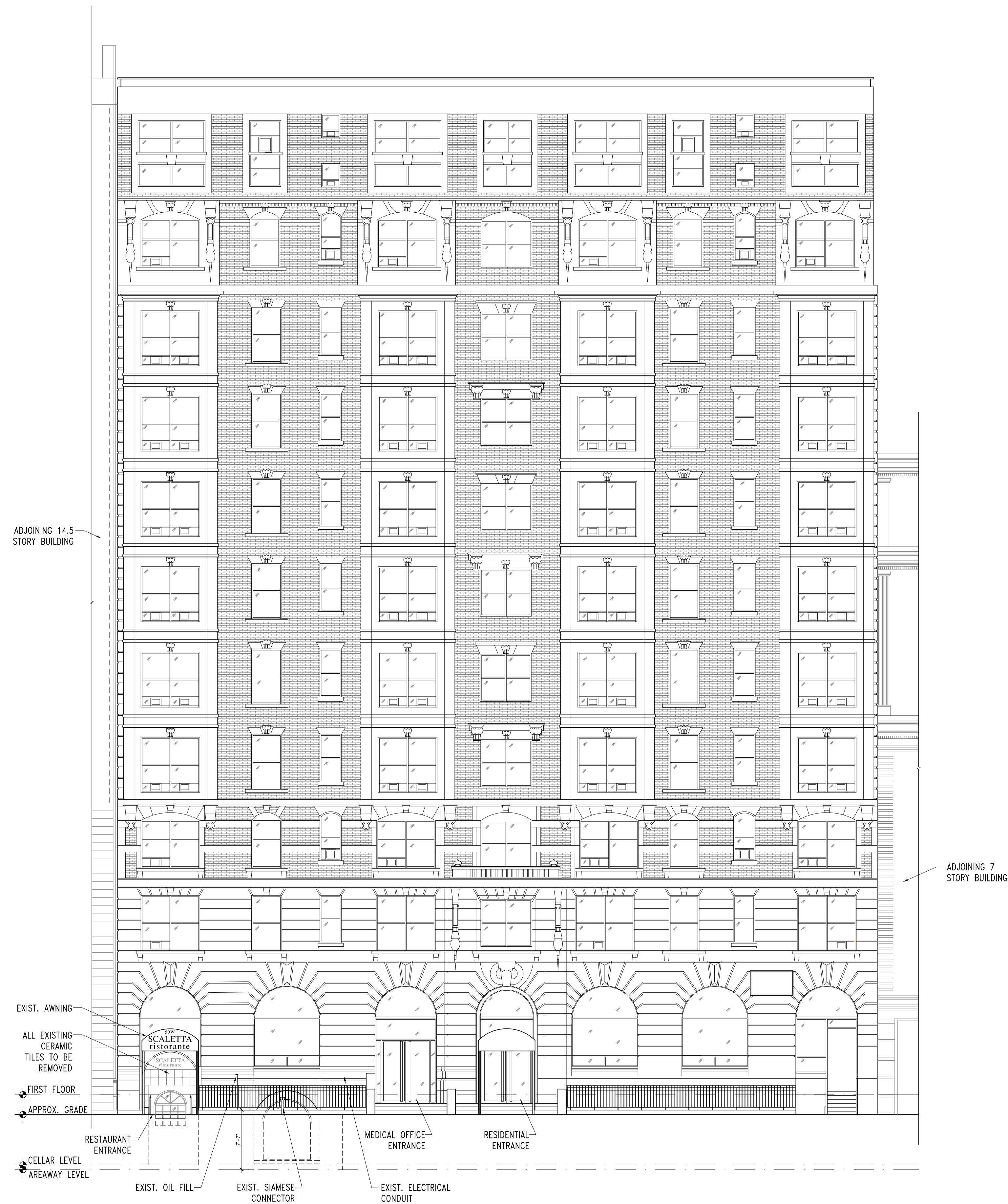
1 EXISTING ELEVATION @ WEST 77TH ST LPC-102 SCALE: 1/8" = 1'-0"
